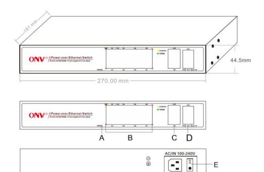
A.Working indicator C.2\*Gigabit Uplink ports E.AC100-240V,50/60Hz
